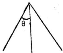
The centre of rotation of the stylus is at the middle of the paper. When the recorder is on its shallowest scale, neglecting the transducer depth adjustment, the transmission mark (zero depth) lies near one edge. The line joining the centre of rotation to the transmission mark then makes an angle of  $\theta = -30^\circ$  with a line parallel to the paper motion.
