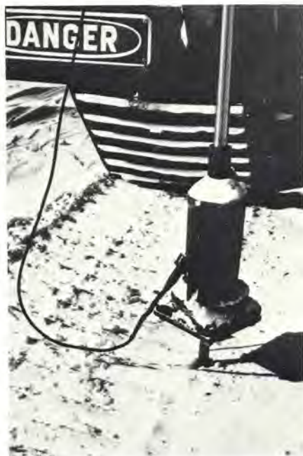
Fig. 5. 3.5/7 KHz transducer and spike in lowered (sounding) position.
