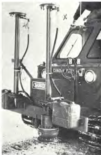
Fig. 3. Front of vehicle and 12/24 KHz transducer.
