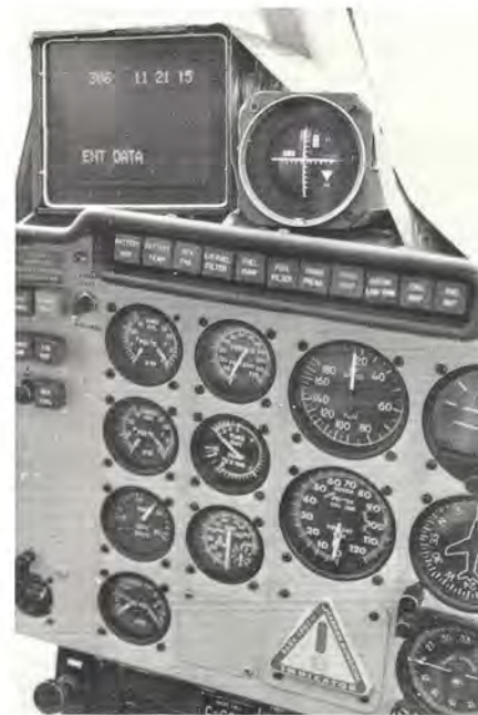
Fig. 18. CRT display and VOR indicator mounted above pilot's console aboard the helicopter
