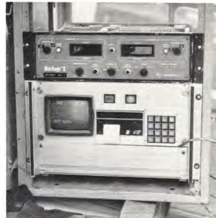
Fig. 17. NavBox and Mini-Ranger III console aboard the helicopter.
