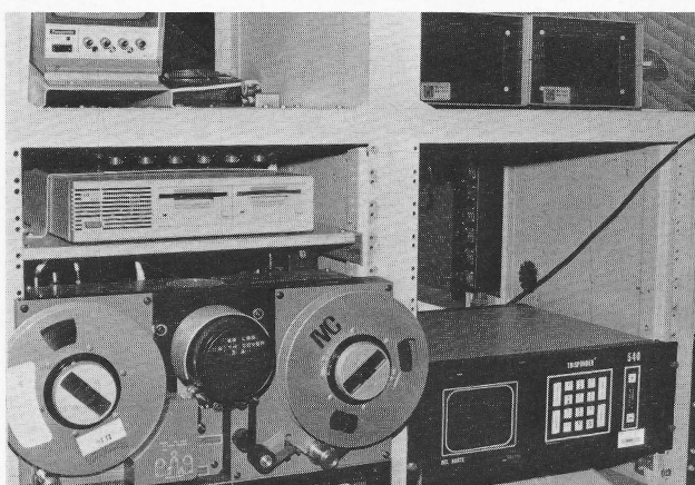
Figure 3: The Trisponder 540 DDMU is seen here on the lower right. To its left is the low-light-level video tape-recorder. Above it is the floppy disc drive (HP9121).
