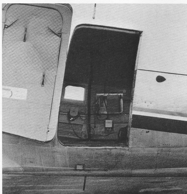
Figure 4: The installation of the Trisponder antennae. Two antennae are used. An antennae switching unit (seen here to the left of the Master R/T) switches back and forth between the two antennae — one mounted through the roof and the other through the floor of the aircraft. Distances are measured to both antennae but only the shorter distance is used. This arrangement alleviates the problem of range-holes and wing-shadowing.
