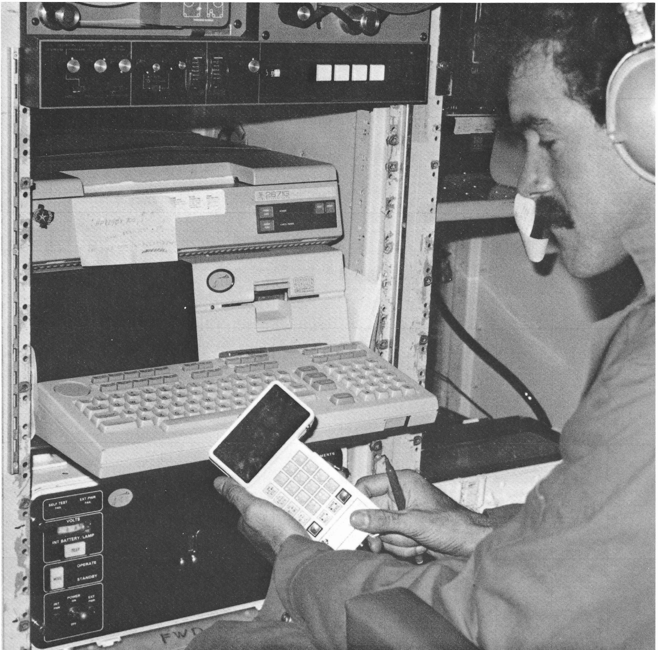
Figure 1: Nortech's Pat Fenton holds the TI4100's Visual Display Unit (VDU) which displays the position via LED's. The actual receiver shown here at the bottom of the rack. Above it lies the HP9826 microcomputer.
