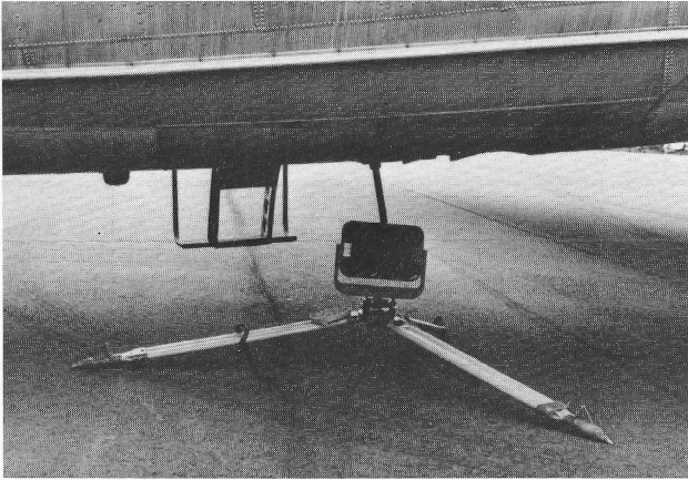
Figure 5: The Trisponder was calibrated daily with a WILD Disto-mat DI20.
