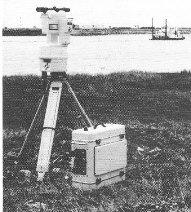
Fig. 1: POLARFIX laser positioning of dredger.
