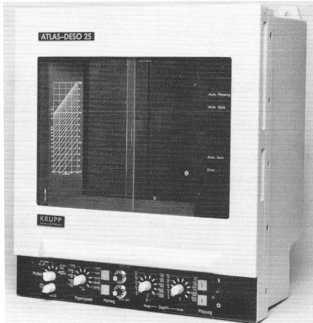
Fig. 6: Sediment and survey sounder DESO 25.
