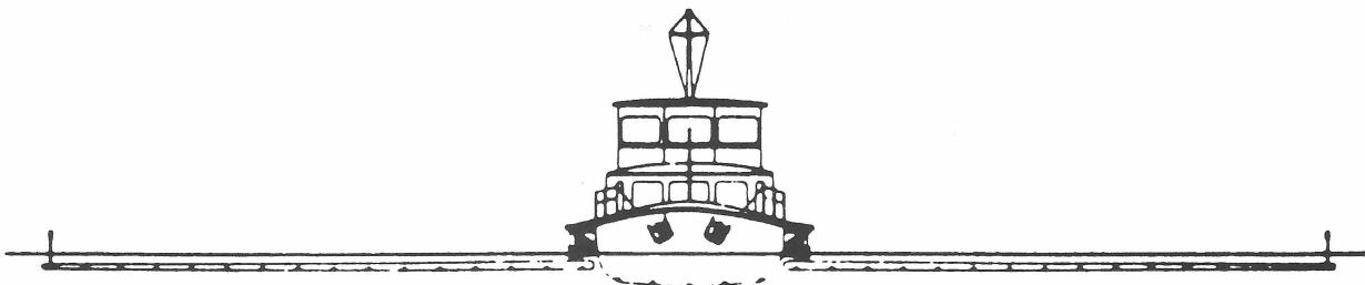
Fig. 3: Swath transducer booms.
