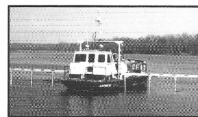
36 foot survey launch with 9 channel sweep.
