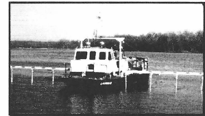
36 foot survey launch with 9 channel sweep.
