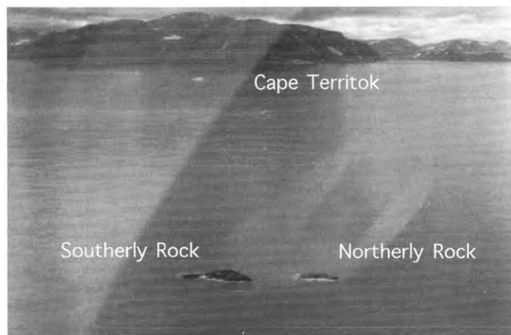
Figure 6. Two, unnamed rocks east of Cape Territok. The southerly rock was part of an EDM traverse in 1973 and is 2.0 m above high water. The northerly one is located at 59° 43' 45"N, 63° 43' 28"W and is 0.5 m above high water.
