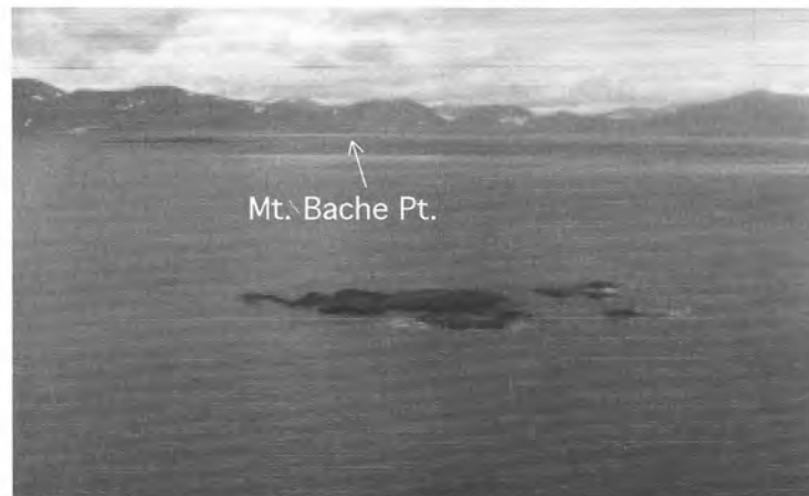
Figure 9. Unnamed rock on the east side of the Galvano Group. The rock was spotted in airphotos. The GPS position of the rock is 59° 55' 30"N, 63° 52' 55"W, which is about 430 m north of the uncontrolled airphoto mosaic position. The rock is 0.5 m above high water. Note the common islands in the middle distance 'moving' relative to the hills in the background of Figures 8 and 9. [Roll 6, #22]
