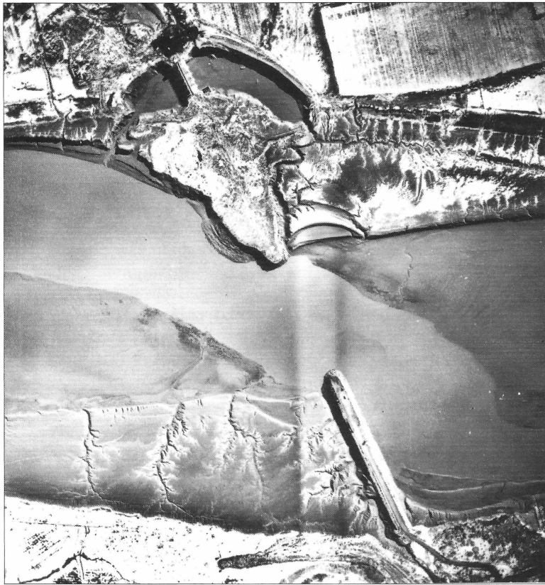
Figure 1: The Petitcodiac River Causeway under construction. Downstream is to the left. The mudflat is growing at the same rate as the causeway is extended.
