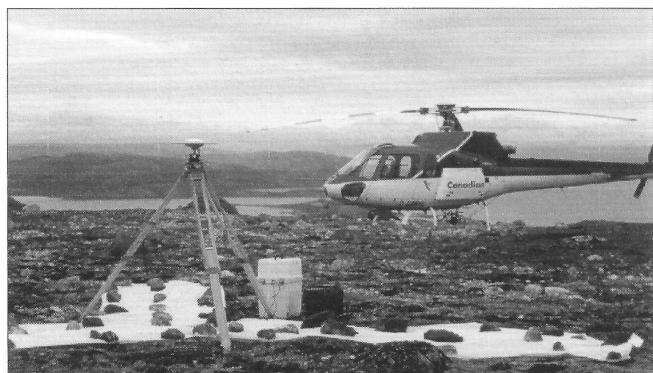
Figure 3 - Ground control established for aerial photography. Okak Bay, Labrador, July 2003.
