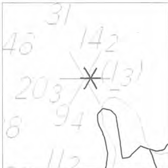
Figure 16 - Gray data from CHS field sheet 1001405 surveyed in September 2003 using Differential GPS. Black data from aerial photograph. Shoreline (black) digitized via contractor; rock (*) digitized by CHS 'rubber sheeting'.
