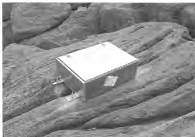
Figure 4 - Example of tide gauge at Brownell Point bolted to a rock outcrop. This gauge was destroyed by polar bears after this picture was taken.
