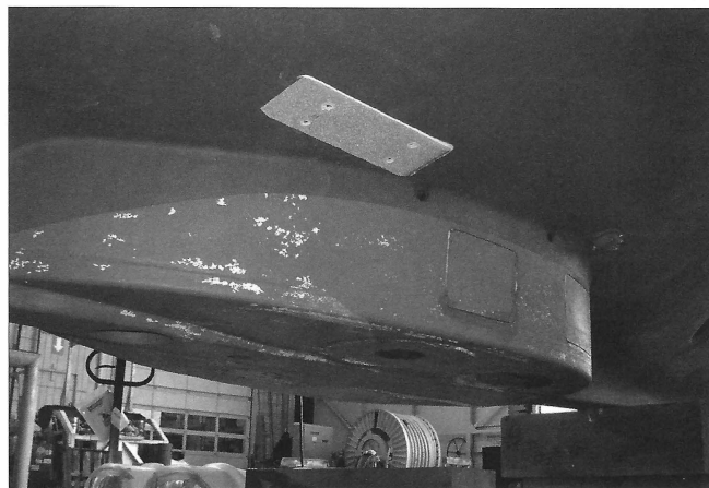
Figure 5: Otter Bay along-keel transducer pod (EM3002 is on port forward).
