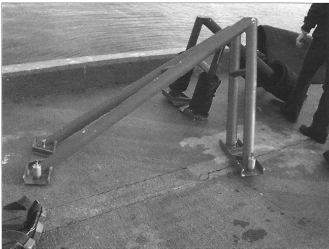
Figure 9: Vector EM1002A transducer protection grids (cow catcher).
