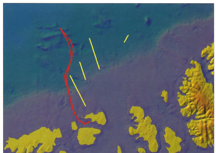
Figure 11: Winter 2010 - AUV survey track in red; helicopter sounding profiles in yellow
