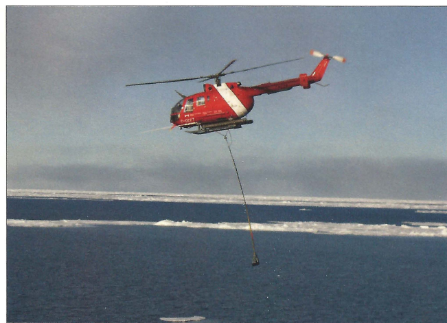
Figure 4: Spot sounding from CCGS Louis S. St-Laurent helicopter
